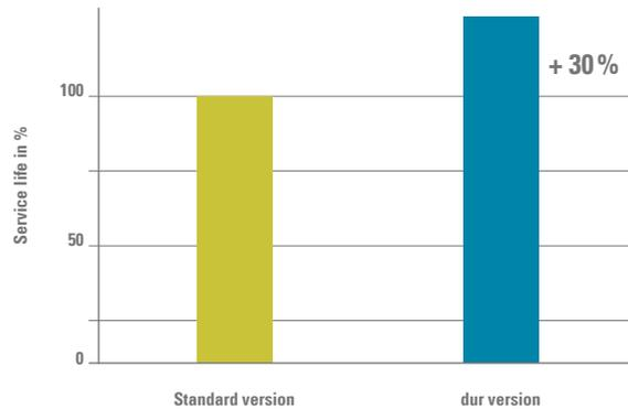
This benefit however can only be fully realized if the needle rotation system is adapted accordingly. If the rotation system is adjusted for this new material, the needles can remain in the board up to 30 % longer than with the standard material, and the product properties remain the same over a longer period of time.
