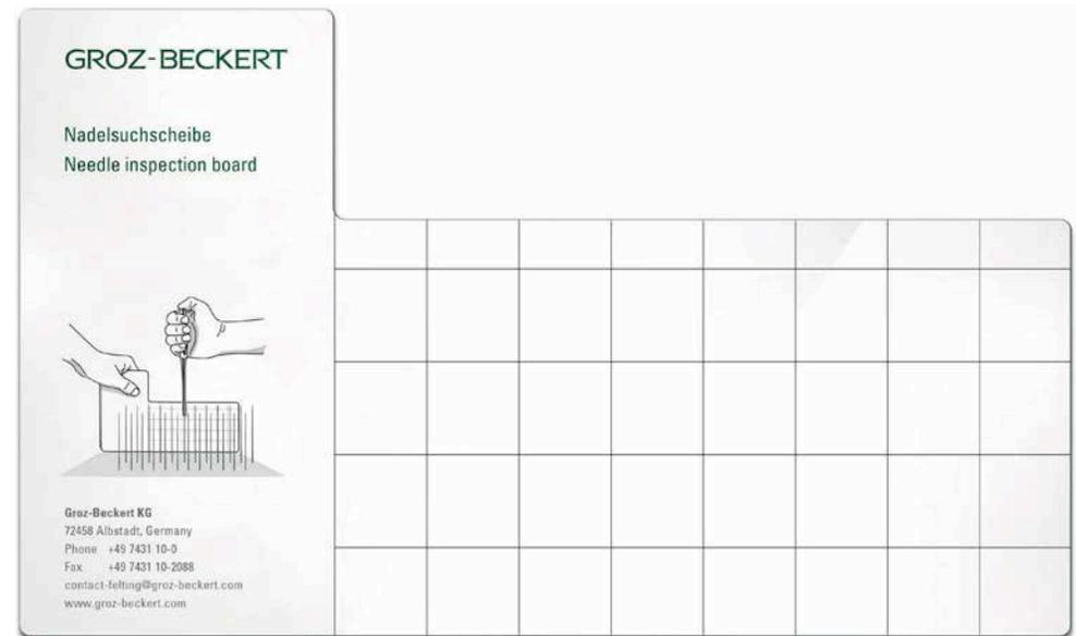
In order to locate broken needles among the large number of needles in the board, the needle inspection board from Groz-Beckert is guided row-by-row through the needles, by the user crosswise to the machine direction. Every needle can thus be checked and broken or damaged needles located and replaced if necessary. Equipped needle boards can also be checked using the needle inspection board to ensure that all needles are aligned correctly. This check can be
